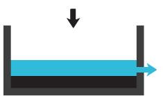
**IDLE:** The idle period is not a designated time frame but rather is that period between completion of decant and beginning of fill. Idle periods occur when actual flows are less than design flows. When idle periods are long, aeration is required to prevent septic conditions from forming.
