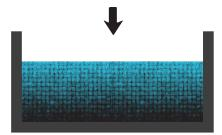
**SETTLE:** One of the major advantages of the SBR system is the creation of "perfect" conditions for the settle period. There is no inflow of waste, no mixing, and no injection of air. A healthy activated sludge floc settles rapidly - in 15-20 minutes. A design time of one hour is most adequate for the settle period.
